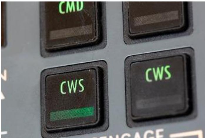
CWS is an acronym for Control Wheel Steering. Broadly speaking, it is a sub-set of the autopilot system which can be used on either System A or B. When engaged, CWS maneuvers the aircraft in response to control pressures applied to the control wheel or column.
